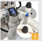
Featuring a wrap-around belt and a counterpressure plate, the machine is suitable for a very wide range of cylindrical products.
