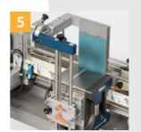
Printing units like hot-foil or thermal transfer printers can be easily integrated.
